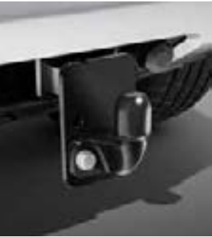
Multi-Height Tow Bar and Armature† VPLWT0159, VPLWB0136 / 37 / 39 Multi-height tow hitch allows for two different tow-ball height positions. Simple to fit, once armature installed, and can be swapped between positions in seconds. 50mm tow ball is included and will take up to 3,500kg trailer load and 200kg nose weight.
