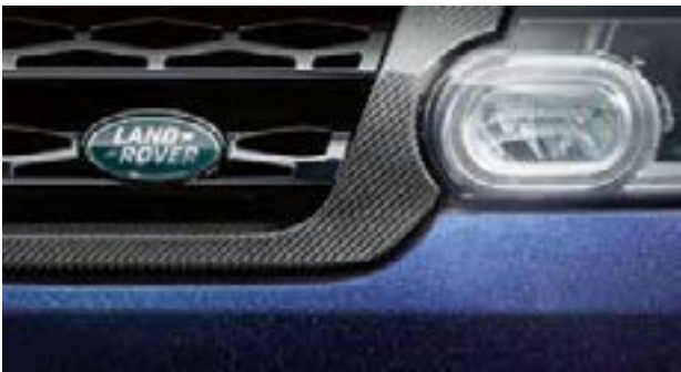
Front Grille Surround – Carbon Fibre* VPLWB0233 High grade Carbon Fibre front grille surround, with a High Gloss finish, provides a premium exterior design upgrade to highlight the dynamic capabilities and performance-inspired design of Range Rover Sport. Fog Lamp Bezel – Carbon Fibre* VPLWB0234 (not shown) High grade Carbon Fibre fog lamp bezel featuring a twill weave and a High Gloss lacquered finish, providing a performance-inspired design enhancement coupled with weight benefits associated with Carbon Fibre.
